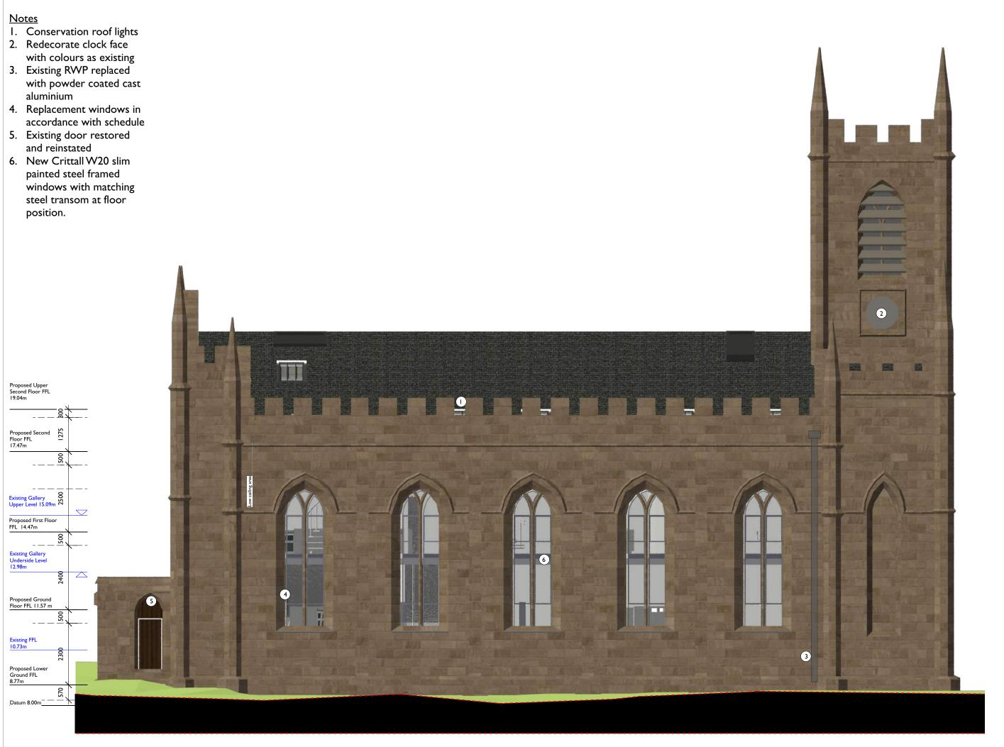
Note: Envelope Repairs Summary: -Damaged and missing stone mullions - generally to be colour matched molding mortar or indent repair with matching stone - to specialist stonemason recommendations.
